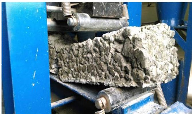
Figure 7 Flexural Test
