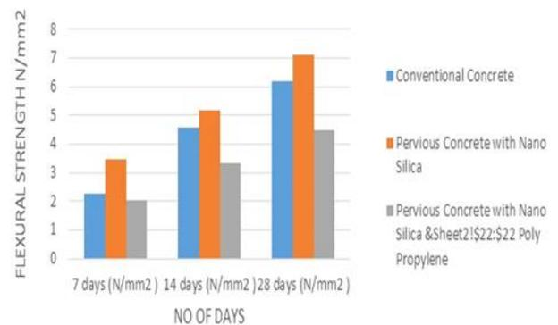
Figure 10 Results for Flexural Strength
