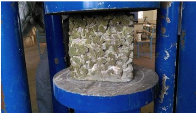
Figure 6 Compression Test
