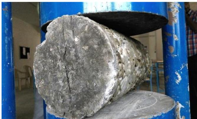
Figure 8 Split Tensile Test
