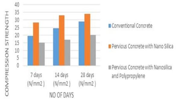
Figure 11 Results for Compressive test
