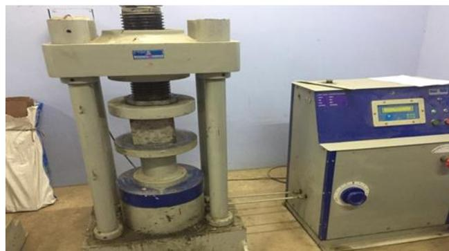
Figure 5 Compressive strength test on the specimen
