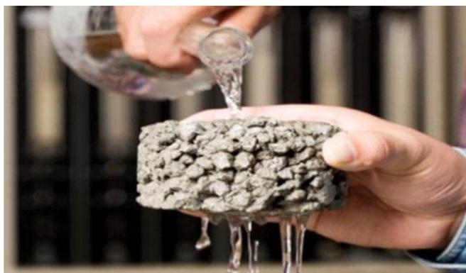
Figure 1 Pervious Concrete
