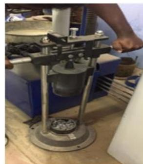
Figure 4 Impact test on aggregate
