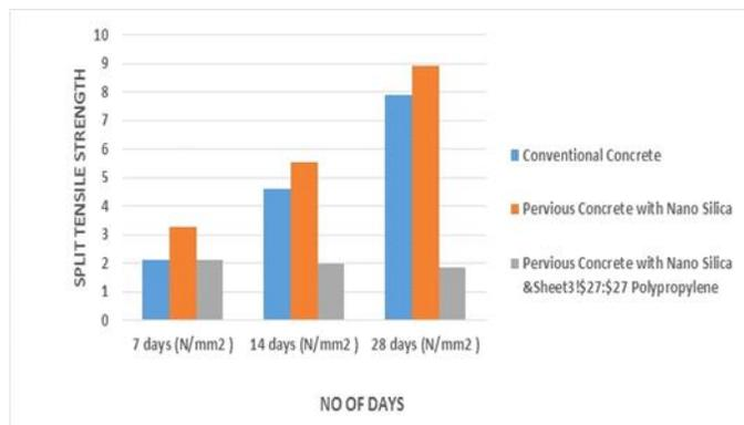
Figure 11 Results for Split Tensile Strength
