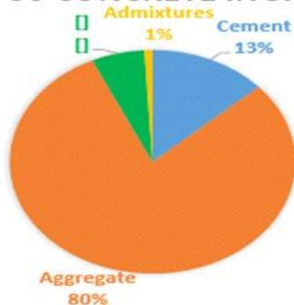
Figure 2 Pervious Concrete Ingredients
